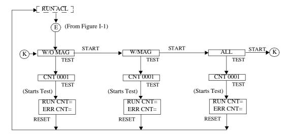
Figure I-3. RUN ACL Flowchart
